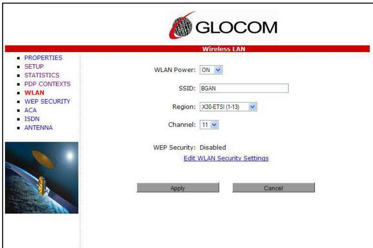
The screenshot displays the GLOCOM web MMI interface for configuring the Wireless LAN. The page title is "Wireless LAN". On the left, a navigation menu lists various settings: PROPERTIES, SETUP, STATISTICS, PDP CONTEXTS, WLAN (highlighted in red), WEP SECURITY, ACA, ISDN, and ANTENNA. Below the menu is a small image of a satellite in space. The main configuration area contains the following settings:
